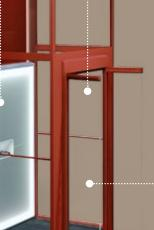
Doors are installed in the lift walls on each floor. The doors are double doors, i.e. two leaves with a central opening. The door leaves are made of glass with painted profiles. LIFT GLASS
